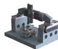
Pick-and-place system with IMS-LM (X,Y), MTN (Z), RV (Rz), BG (Rx,Ry)
